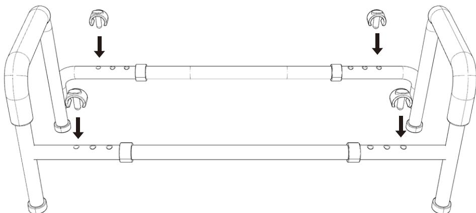
**3. Install the four legs. And adjust buttons on the same level to keep balance.**
